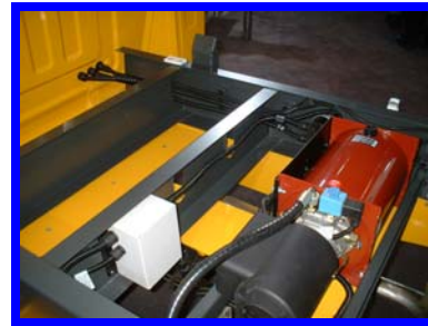
VFS01-11-069 Tipper control system Ford Motor Company
